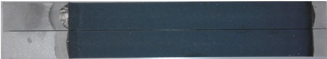
Figure 55: Typical failure surfaces of a DCB specimen tested under mode I in a dry environment.
