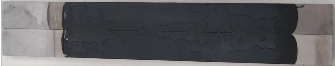
Figure 59: Typical failure surface of the DCB specimens with an adhesive layer of 0.4mm thickness tested under mode I loading in a 0% RH environment.
