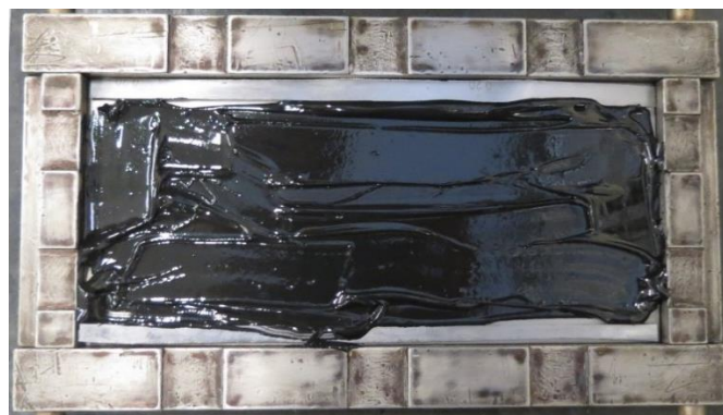
Figure 37: Mould with the adhesive SikaPower®-4720.
