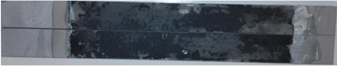
Figure 78: Typical failure surfaces of the ODCB specimens tested under mode I with an adhesive plate aged in a 100% RH environment.
