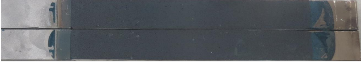
Figure 75: Typical failure surface of the ODCB specimens tested under mode I with an adhesive plate aged in a 75% RH environment.
