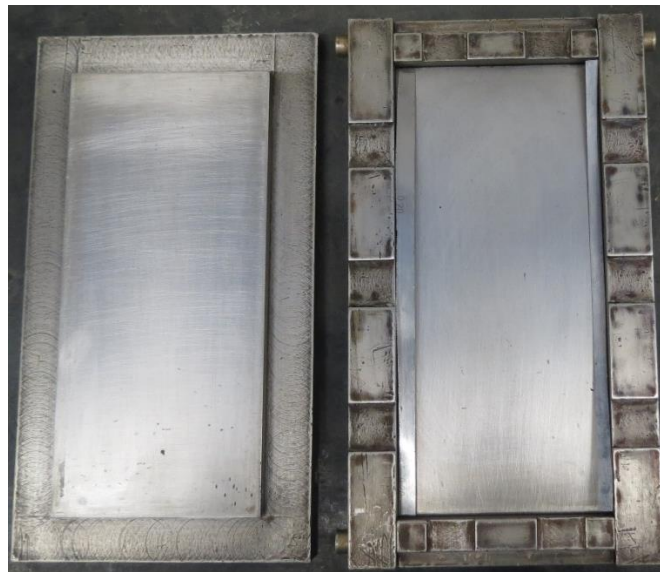
Figure 36: Mould used to produce adhesive plates.
