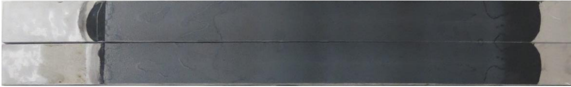
Figure 91: Typical failure surface of the DCB specimens tested under mode II in a 0% RH environment.
