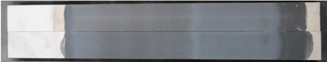
Figure 83: Typical failure surfaces of the DCB specimens tested under mixed-mode 55° loading in a 0% RH environment.
