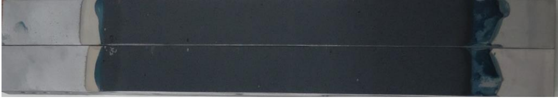
Figure 63: Typical failure surface of an ODCB specimen tested under mode I with a dry adhesive plate.
