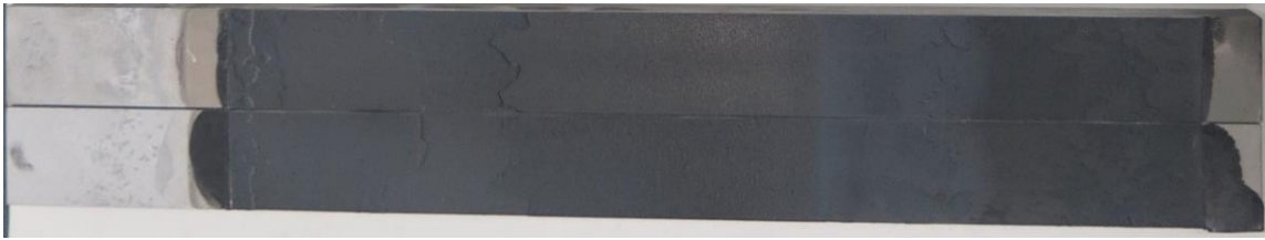
Figure 87: Typical failure surfaces of the DCB specimens tested under mixed-mode 87° in a 0% RH environment.
