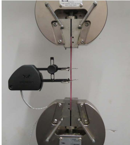
Figure 40 - Apparatus for the bulk tensile testing
