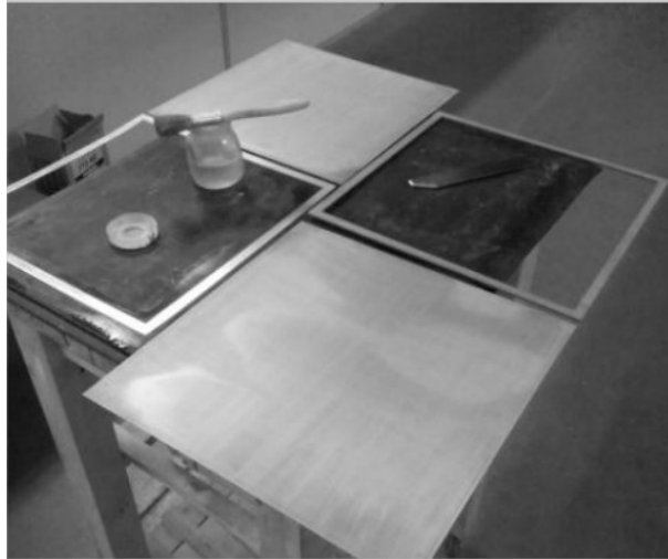
Figure 24 - Drying of the mould releasing agent
