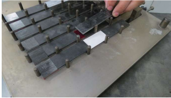
Figure 39 - Bonding of the SLJ in the mould with the spacers already in place
