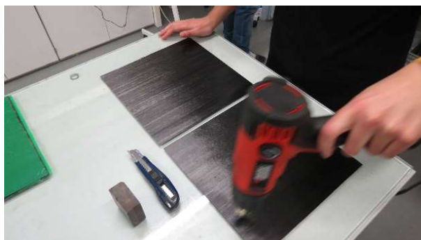
Figure 25 - Pre heating of the CFRP pre-preg layers
