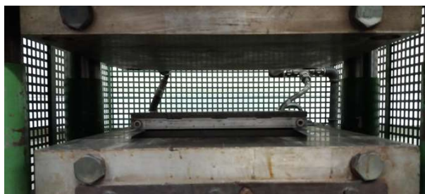
Figure 30 - Mould inserted into the hot plates press
