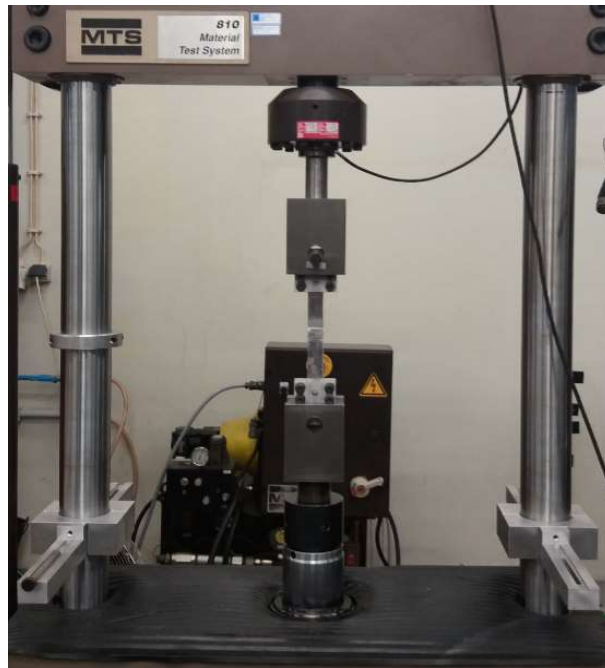
Figure 52 - Apparatus for the SLJ tensile testing
