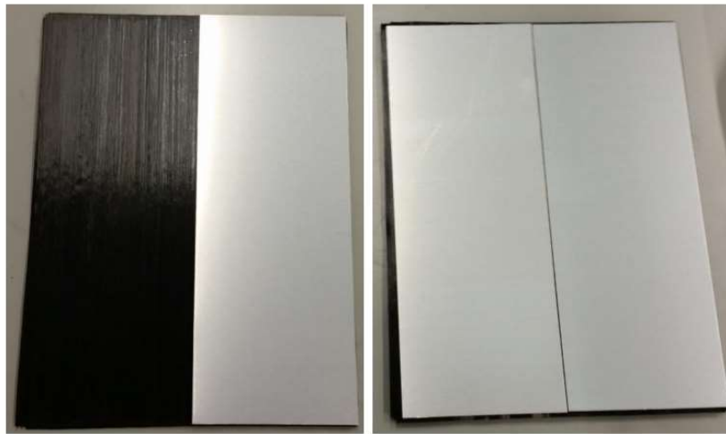
Figure 35 - Stacking of the aluminium sheets over the CFRP laminate
