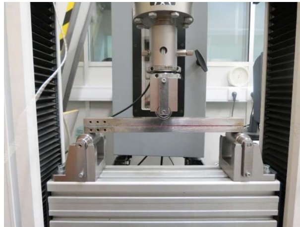
Figure 48 - Apparatus for the ENF test
