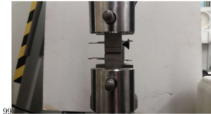
Figure 42 - Apparatus for the TAST test
