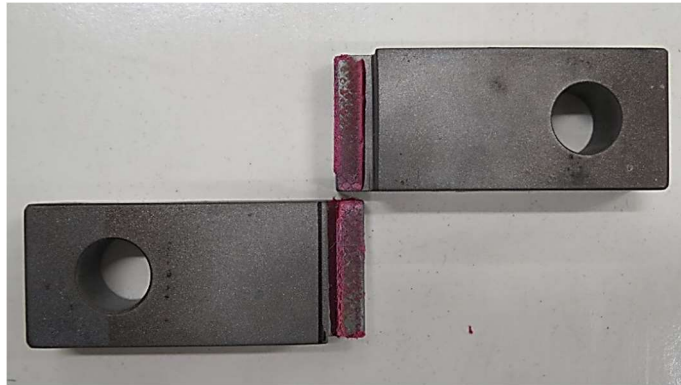
Figure 43 - Fracture surface of a TAST specimen after testing
