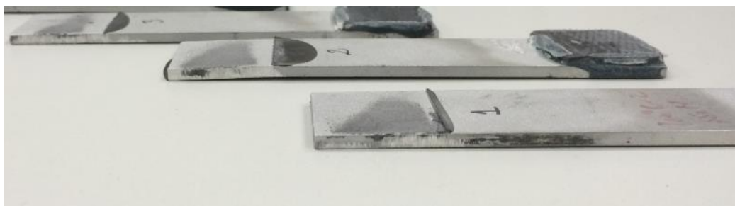
Figure 3.37 Plastic deformation of the 3 mm thick aluminum adherends
