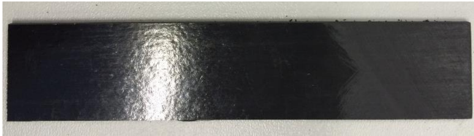
Figure 3.6 CFRP substrate abraded
