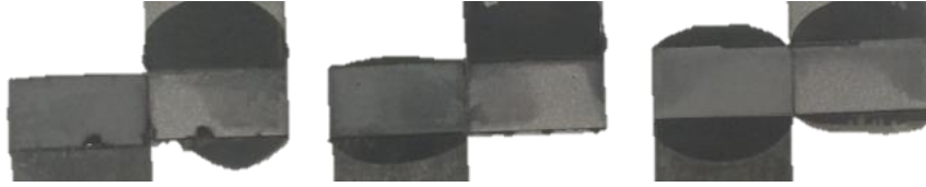
Figure 3.13 Failure modes of CFRP (2.1 mm)/HSS (1 mm) 12.5 mm overlap SLJs tested specimens
