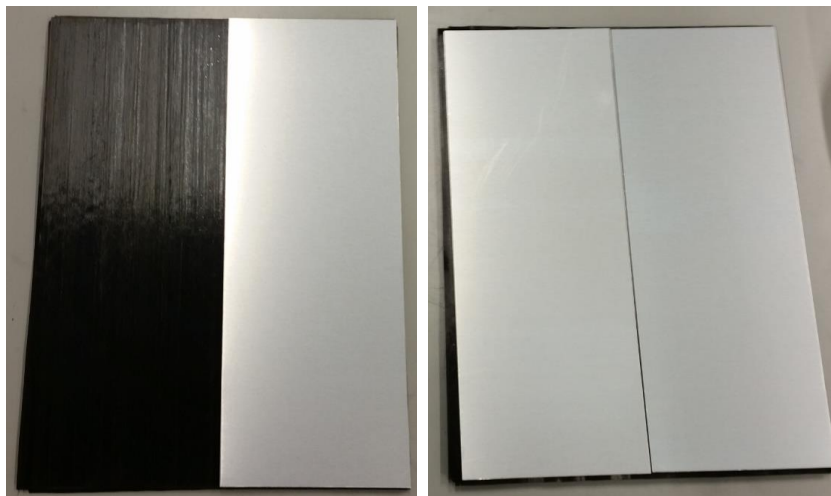
Figure 20 – Laying up the aluminium sheets, one by one
