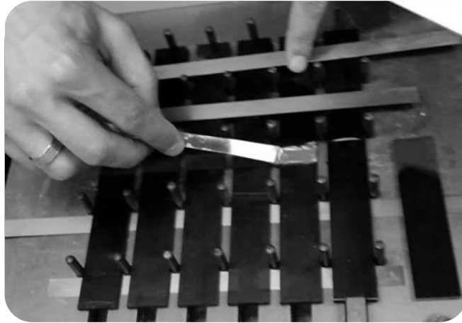
Figure 25 – Application of the adhesive
