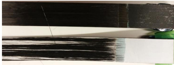
Figure 34 – Failure surface of the peel specimen with pre-crack
