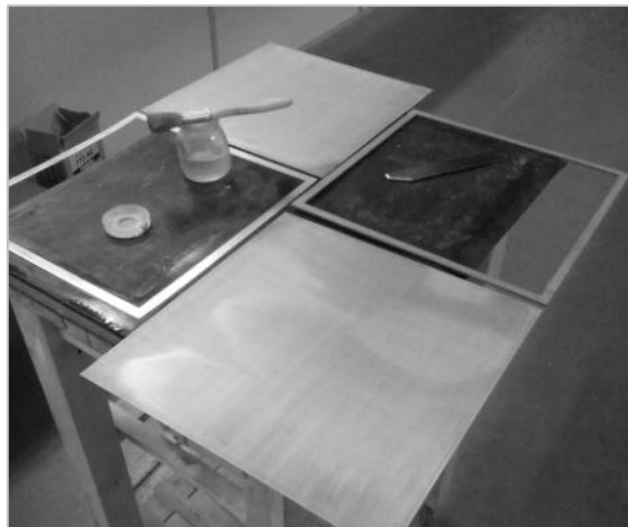
Figure 50- Application of release agent in the metallic sheets.
