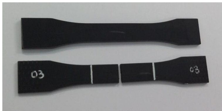
Figure 36- SikaPower 4720 bulk specimens before and after of the tensile test.
