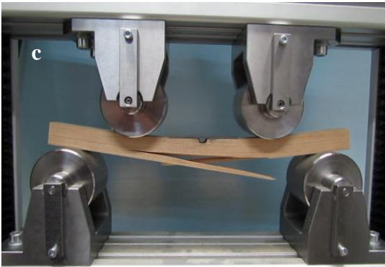
Figure 62: Failure mechanisms observed in the repaired compression damage specimens:
