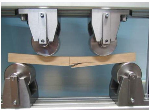
Figure 67: Failure mechanism of an unrepaired cross grain tension specimen
