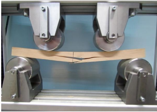
Figure 70: Failure mechanism of a repaired cross grain tension specimen.
