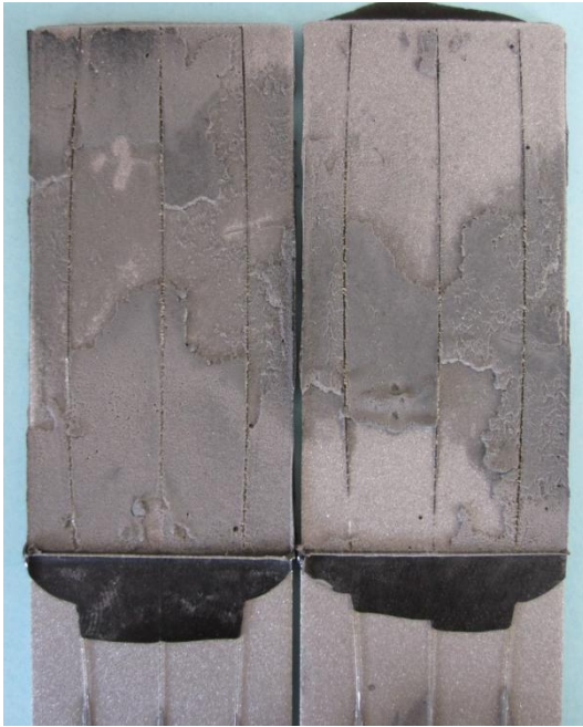
Figure 34- Fracture surface of a joint (fourth trial).
