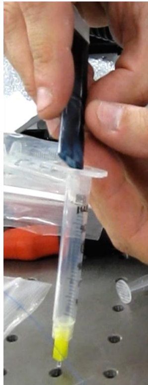
Figure 52- Epoxy is poured into the syringe.
