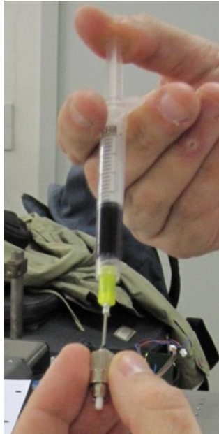
Figure 53- Add epoxy to the connector.
