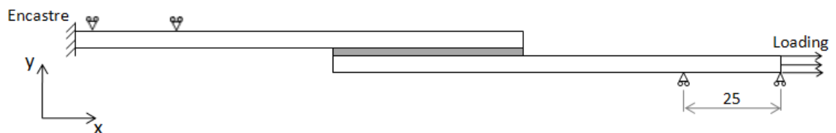
Figure 63- Boundary conditions of the finite element model (not to scale, dimensions in mm).
