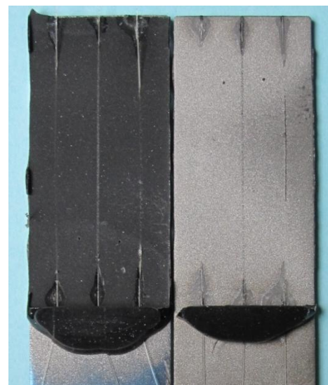
Figure 22- Fracture surface of a joint with fibers (first trial).
