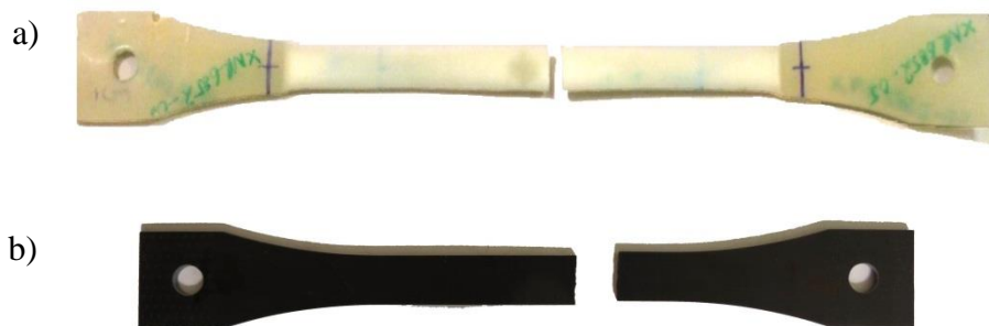
Figure 23 – Bulk tensile specimens after test, a) XNR 6852 and b) SikaPower 4720
