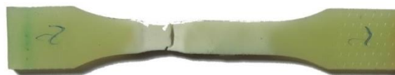
Figure 30 - Ductile fracture of short specimen (25 radius) in the necking part of the specimen using XNR 6852.
