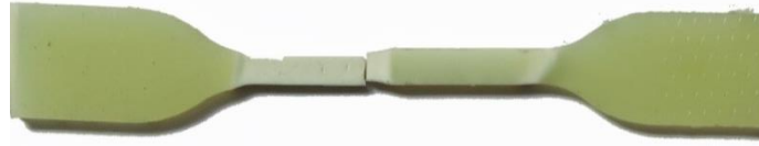
Figure 28 – Ductile fracture of the short specimen (EN ISO 527-2 standard) in the necking part of the specimen using XNR 6852
