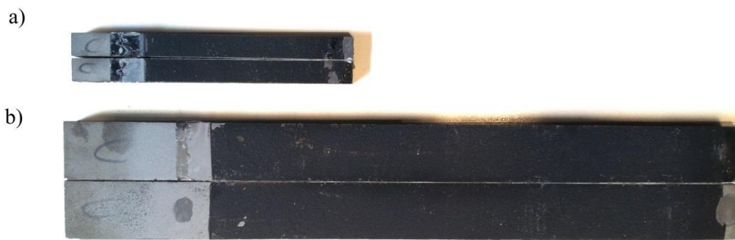
Figure 70 - Two examples of the cohesive fracture surface of the specimens tested, a) small specimen and b) normal specimen.
