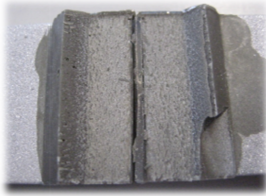
FIGURE 38- AV138 45 DEGREES TAPER FRACTURE SURFACE
