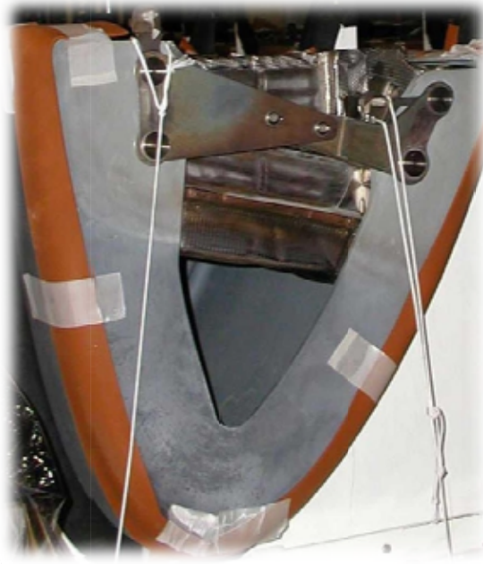
FIGURE 8 - CARBON-CARBON PLATE MOUNTED IN TITANIUM INSERT (18)
