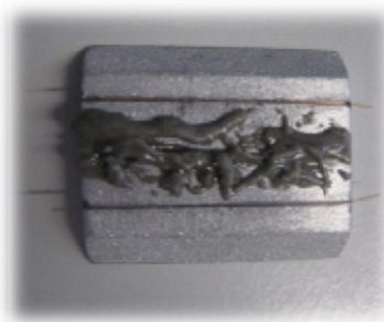
FIGURE 29- BARRIER USED IN DUAL ADHESIVE JOINT CONSTRUCTION
