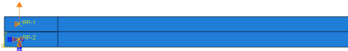
Figure 11: Boundary conditions for the DCB test simulation for quasi-static and intermediate speed.
