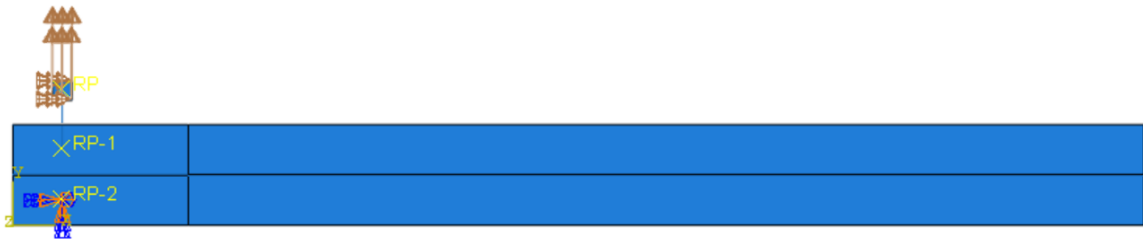
Figure 12: Boundary conditions for the DCB test simulation for impact conditions.
