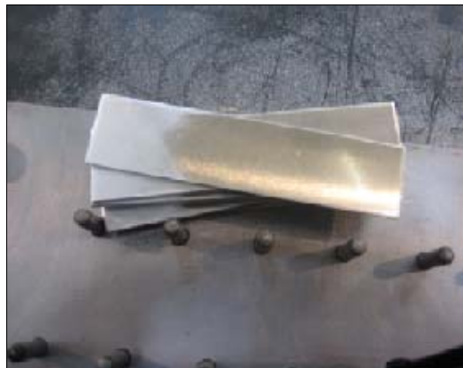
Figure 26 – Sandblasted substrates for SLJs.
