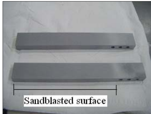
Figure 36 - Sandblasted surface in the substrates.
