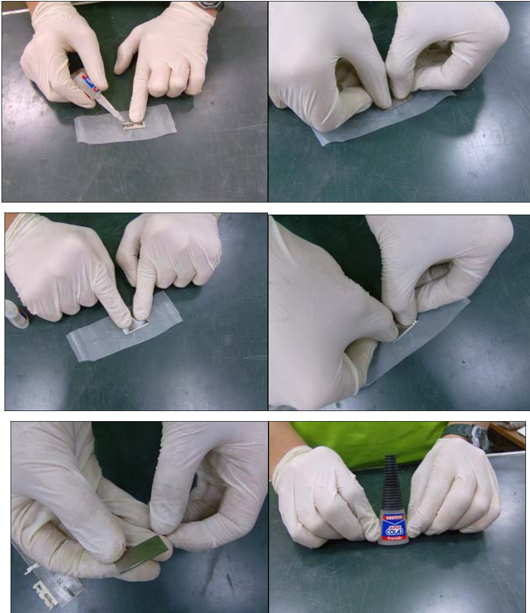
Figure 39- Operation of razor blade spacer bonding.
