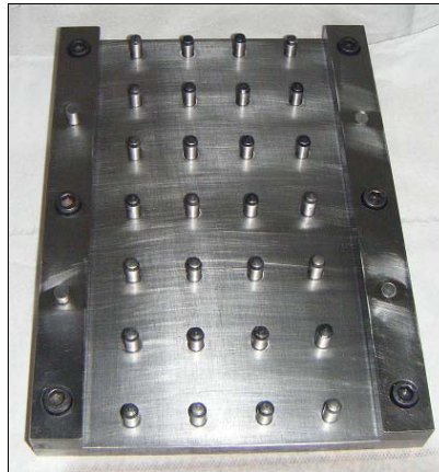
Figure 15- Mould used to produce TAST specimens.
