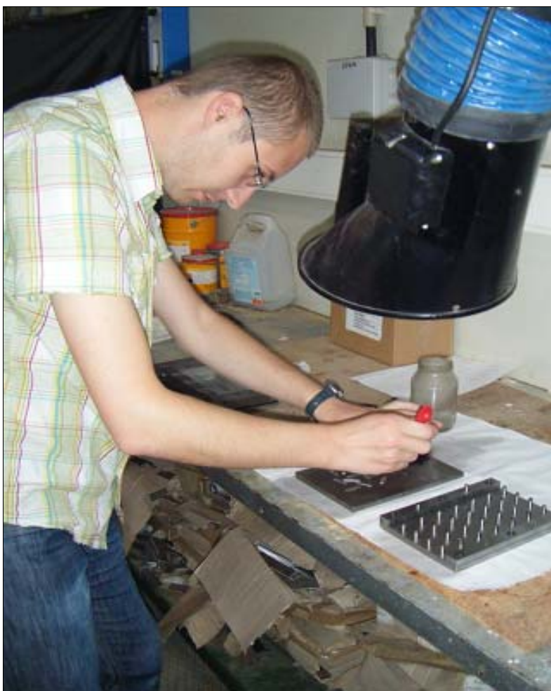
Figure 20 - Application of release agent in a ventilated place.
