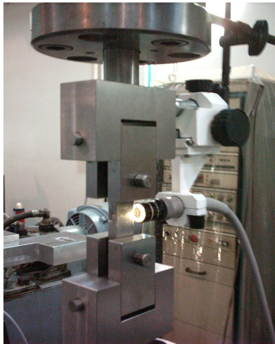
Figure 43 – TAST specimen set-up.
