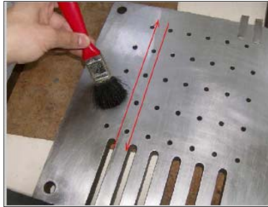
Figure 27 – Release agent application to the SLJs mould.
