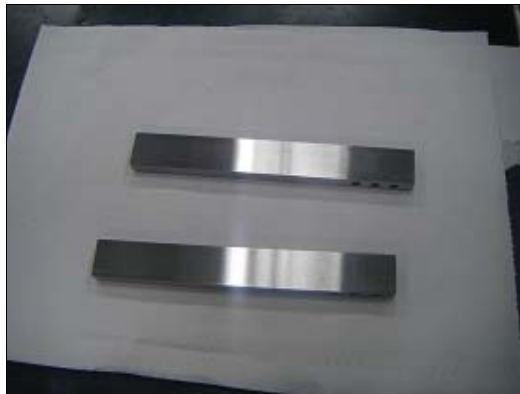
Figure 35- Steel substrates used for DCB test.
