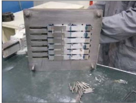
Figure 32 - Mould pin removal.
