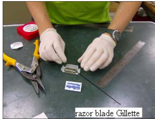
Figure 37 - Razor blades used to promote the initiation of the crack.
