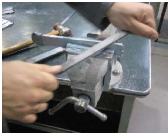
Figure 33 - Adhesive removal with a small woodworking file.
