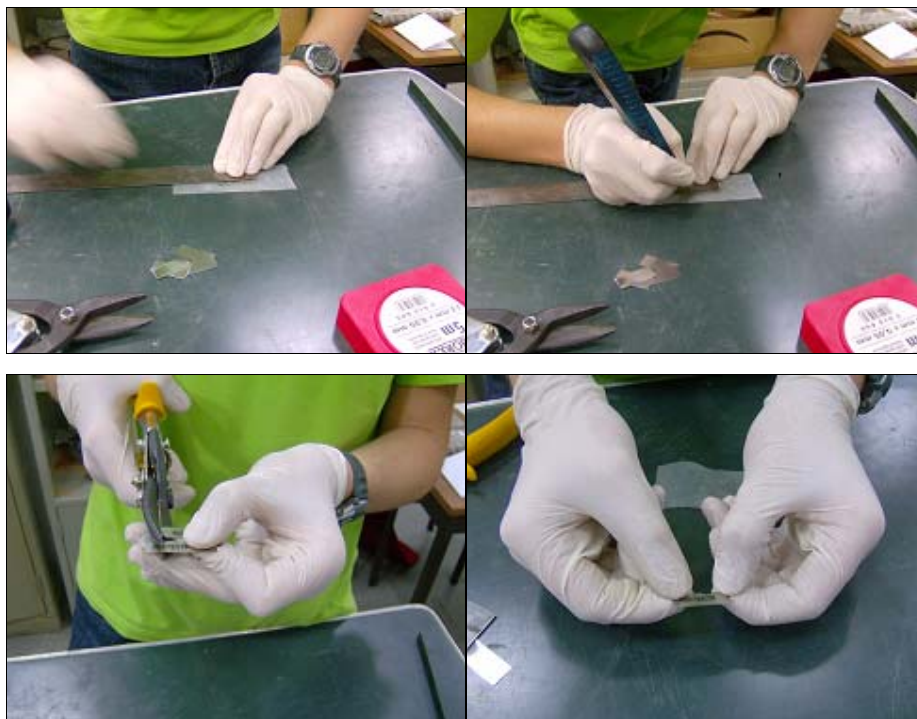
Figure 38 –Measuring and cutting of the razorblade in two symmetric blades.
