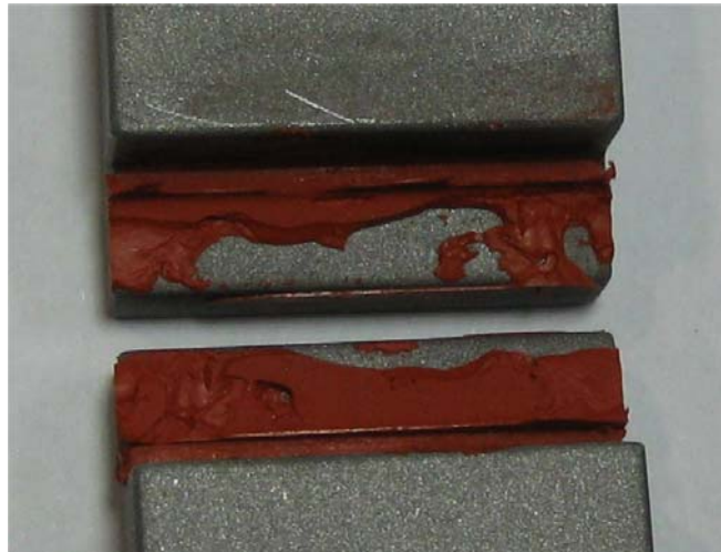
Figure 47 - Failure mode in TAST specimens.
