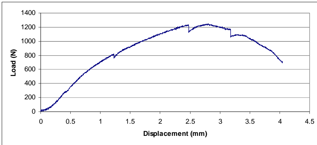
Figure 50 - Typical DCB load-displacement curve
