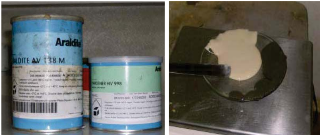
Figure 39 – a) Adhesive AV138M and hardener separate containers and b) mixture tools to mix the two components.
