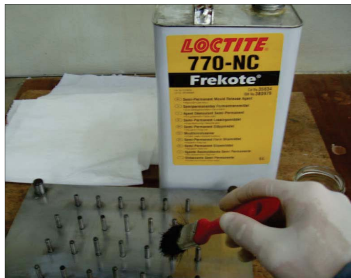
Figure 31. Mould release agent application
