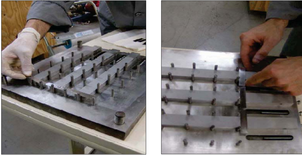
Figure 36. Application of the top spacers (gauge feeler in the left and razorblade assembly in the right).
