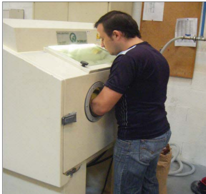
Figure 33. Working with the sandblaster
