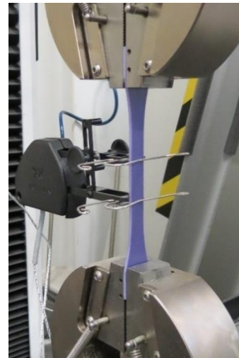
Figure 28 - a) Tensile curve [23], b) tensile test using an extensometer.
