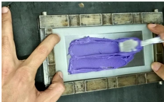
Figure 25 - a) Application of adhesive to a bulk mold, b) closing the bulk sheet mold applying a basculation technique.
