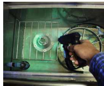
Figure 2.6: Removal of the excess liquid from the surface.
