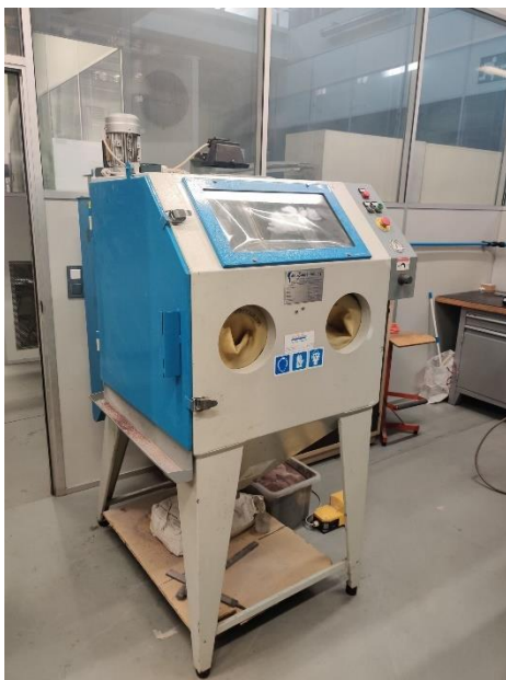
Figure 3.2: Shot blasting machine used.
