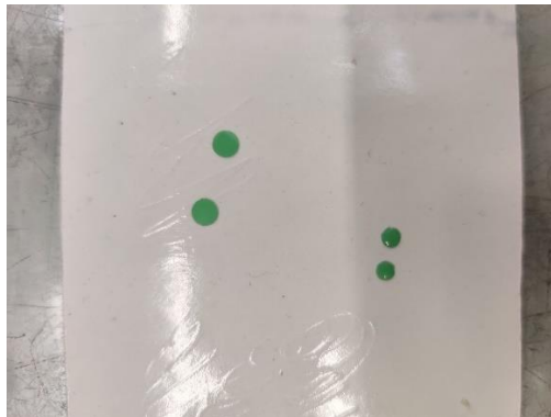
Figure 3.5: Teflon fibre circles used to generate the void in the SLJ.
