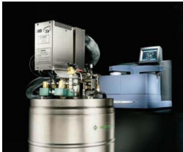
Figure 2.12 - LNCS cooling system refrigerating the chamber of a DSC Q2000 (Dallas and Aubuchon, 2016).
