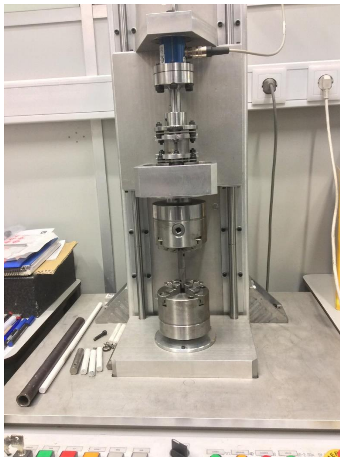
Figure 1.2 - Torsion machine that determines adhesive shear properties.
