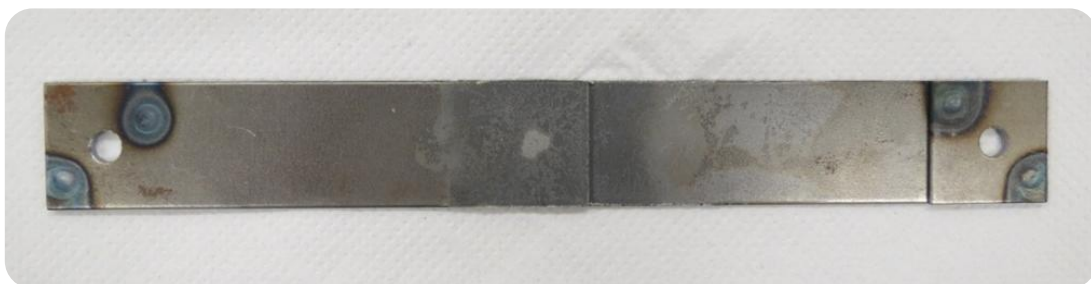
Figure 27. SLJ specimen manufactured for impact tests.
