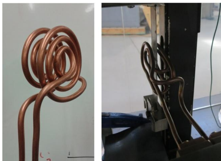
Figure 34. Induction coils manufactured (pancake shape at left and U-shape at right).
