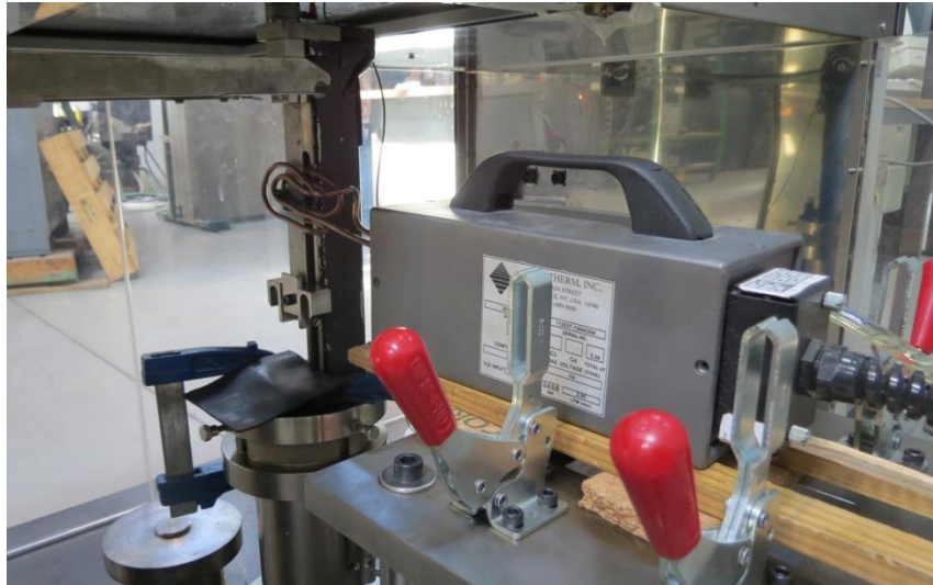
Figure 35. Heating of the specimen for the impact test at high temperature.
