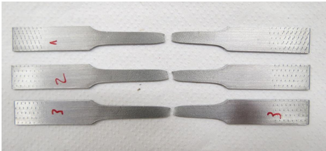
Figure 50. Fracture mode of the steel specimens tested.
