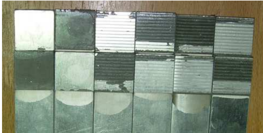
Figure 24 Fracture surfaces of specimens bonded with AV138 without chemical surface treatment. The surface patterns from left to right are: no surface pattern, 0.1 mm at 90° and 0.3 mm at 90°
