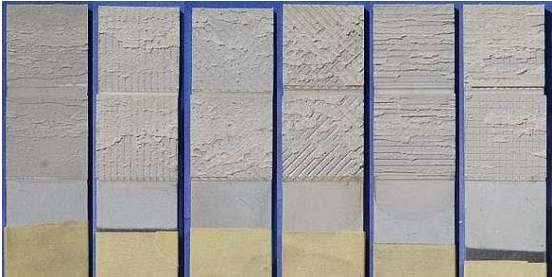
Figure 39 Fracture surfaces of specimens bonded with Araldite 2015 with chemical surface treatment. The surface patterns from left to right are: no surface pattern, 0°, 45°, 45° crossed, 90° and 90° crossed [13]
