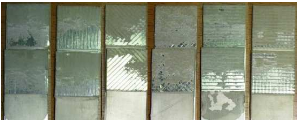
Figure 37 Fracture surfaces of specimens bonded with Araldite 2015 without chemical surface treatment. The surface patterns from left to right are: no surface pattern, 0°, 45°, 45° crossed, 90° and 90° crossed
