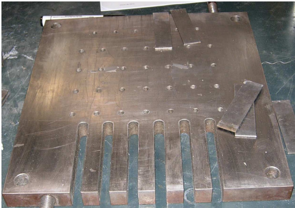
Figure 18 Top half of the mould used for the manufacturing of the adhesive joints
