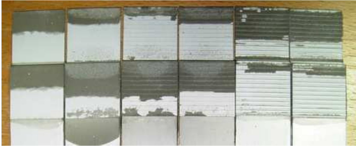
Figure 26 Fracture surfaces of specimens bonded with AV138 with chemical surface treatment. The surface patterns from left to right are: no surface pattern, 0.1 mm at 90° and 0.3 mm at 90°
