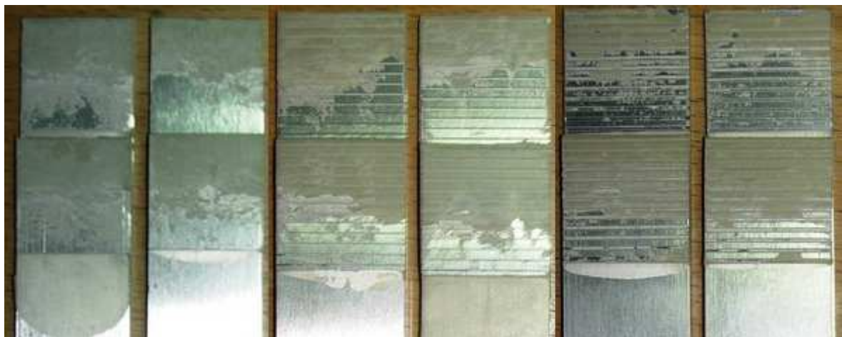
Figure 28 Fracture surfaces of specimens bonded with Araldite 2015 without chemical surface treatment. The surface patterns from left to right are: no surface pattern, 0.1 mm at 90° and 0.3 mm at 90°
