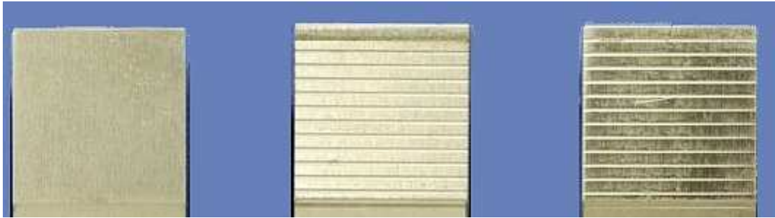
Figure 15 Specimens with no pattern and a 90° pattern with depths of 0.1mm and 0.3mm
