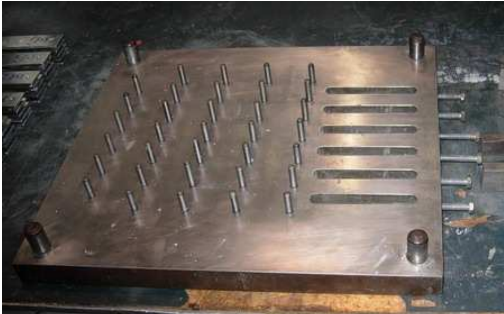
Figure 17 Bottom half of mould used for the manufacturing of the adhesive joints
