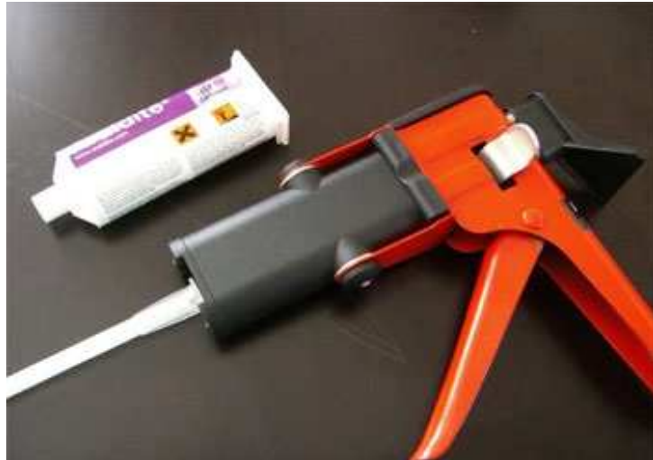
Figure 11 Araldite 2015 with dual syringe dispensing system
