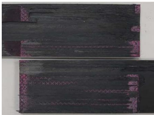
Figure 44 - Typical failure surface of 50 mm overlap CFRP-only SLJs
