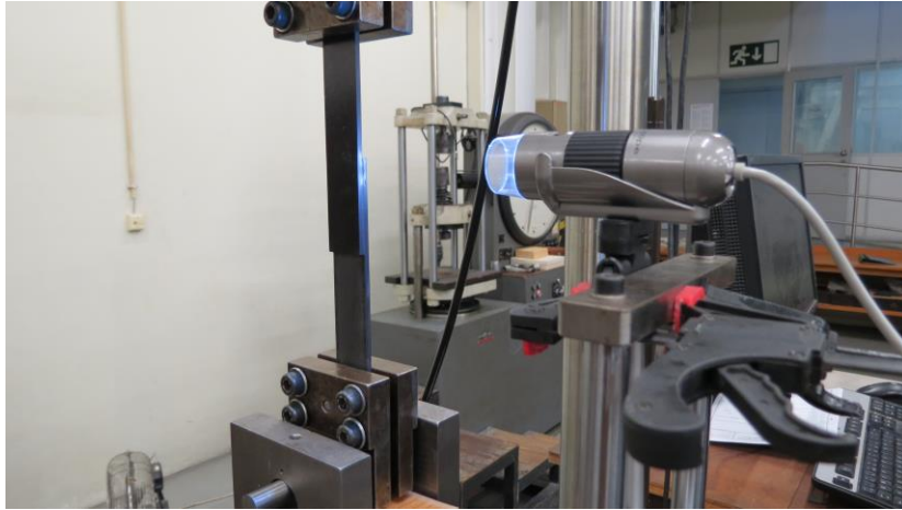
Figure 40 - Video system setup to observe the delamination phenomenon
