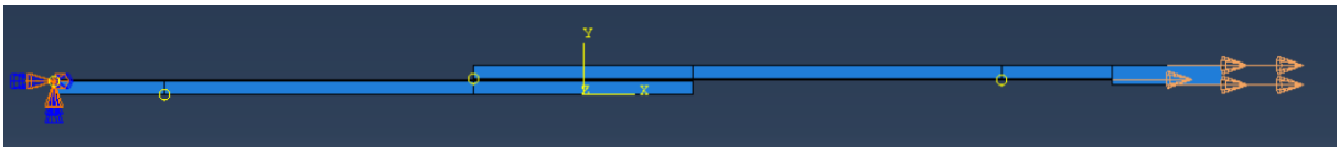
Figure 85 - Schematic view of the physical boundary conditions for SLJs under impact conditions in Abaqus®
