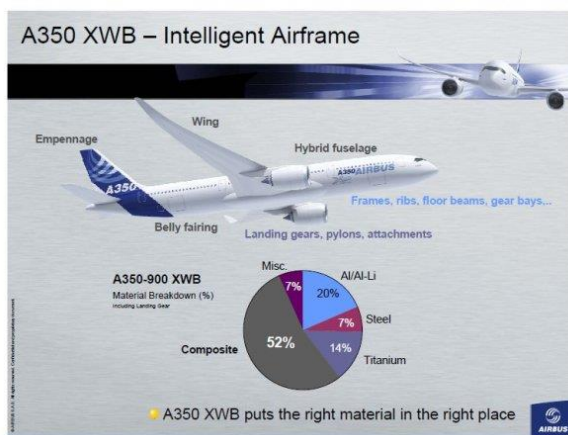
Figure 1 - Composition of A350 XWB [4]
