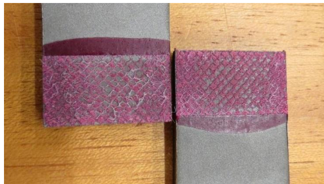
Figure 50 - Typical failure surface of 12.5 mm overlap Ti-CFRP SLJs
