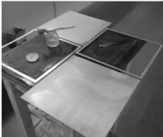
Figure 26 - Application of releasing agent to the mould components
