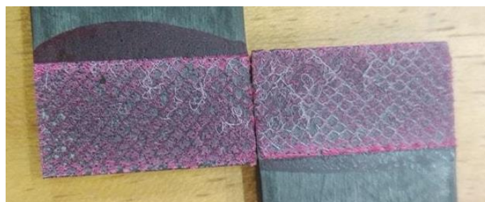
Figure 42 - Typical failure surface of 12.5 mm overlap CFRP-only SLJs
