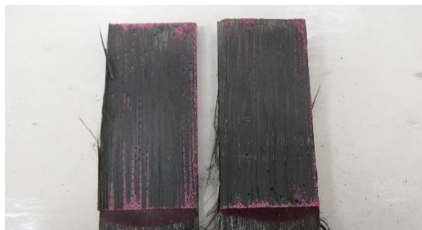
Figure 48 - Typical failure surface of 50 mm overlap CFRP-Ti-CFRP SLJs
