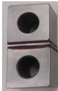
Figure 31 - Bonding between the steel blocks and the specimen CFRP-Ti-CFRP
